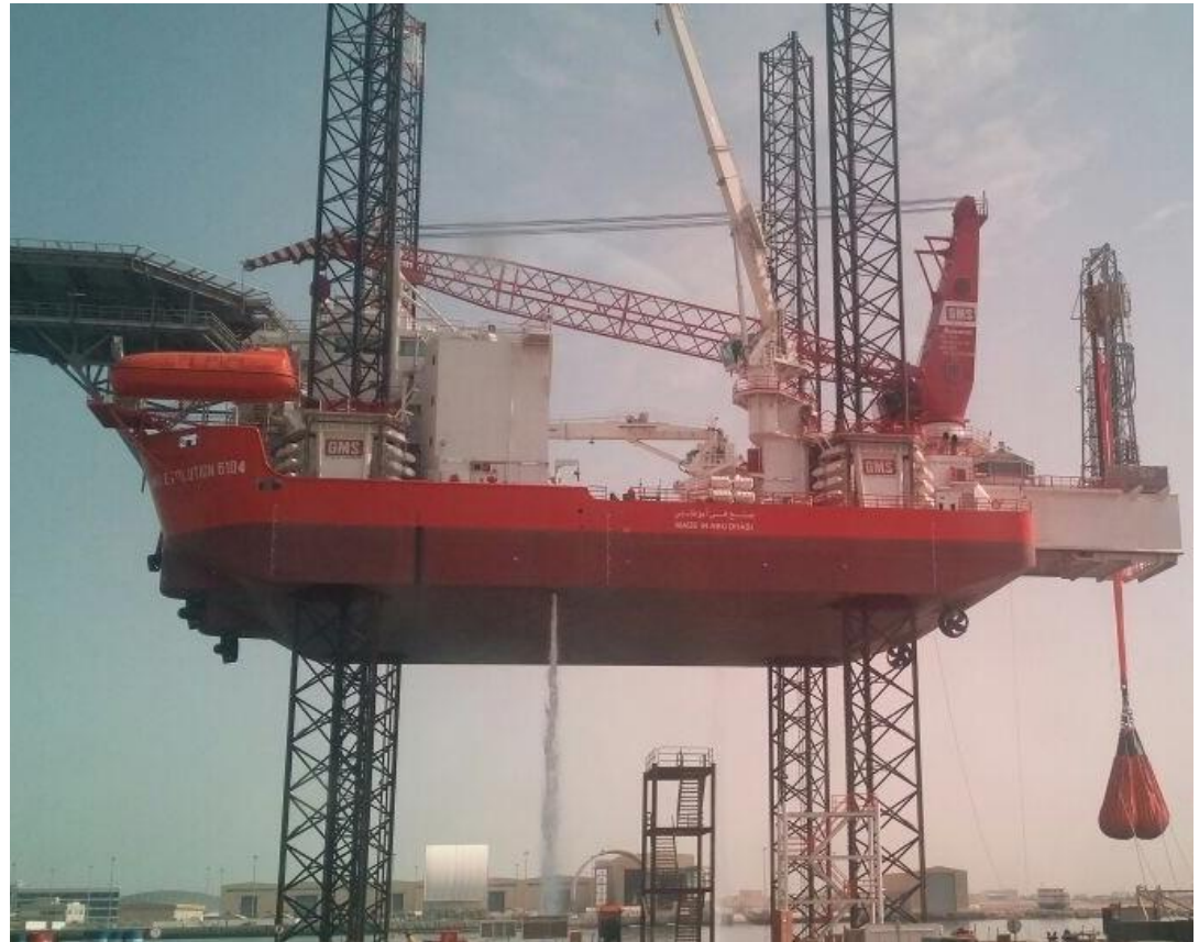
GMS Evolution's cantilever load testing to 250 tonnes
